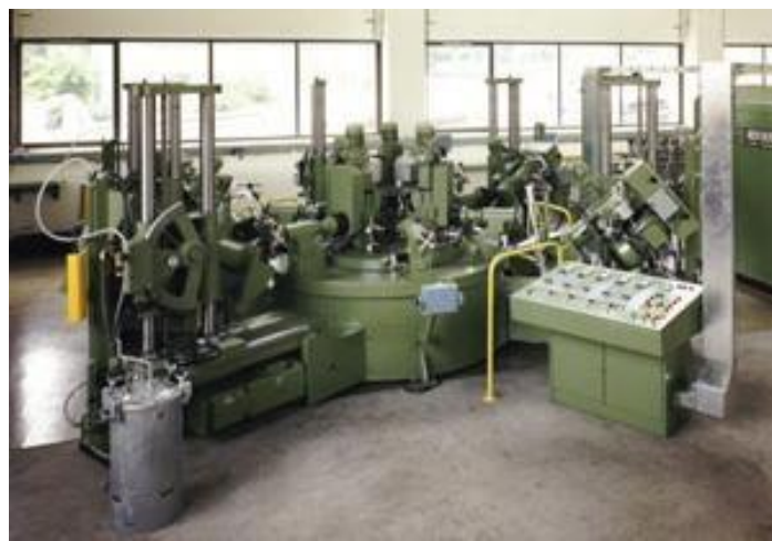
Figure 1.16 Example of 6 station rotary configuration
