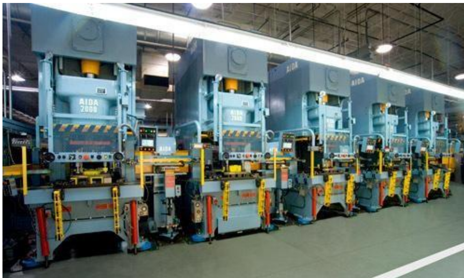
Figure 1.29 Example of 20 stations Transfer line
