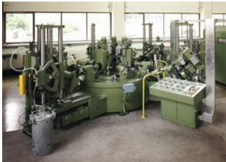
Figure 1.26 Example of 6 station rotary configuration
